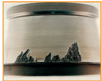
Geometric stress concentration — Spalling from misalignment, deflections or heavy loading.
