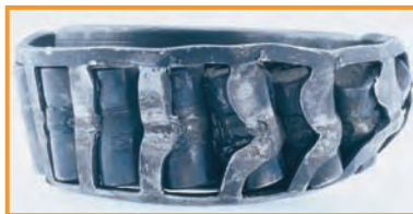
Total bearing lock-up — Rollers skew, slide sideways and lock-up bearing.
