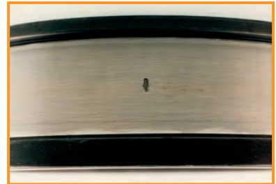
Inclusion origin — Spalling from oxides or other hard inclusions in bearing steel.
