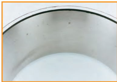
Roller spaced nicking — Raised metal on races from contact with roller edges.
