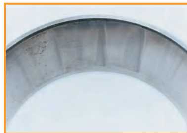
Scalloping — Uneven localized wear resulting from excessive end play.
