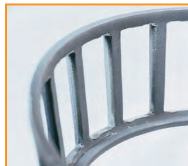
Cage pocket wear — Heavy contact between the rollers and cage pocket surfaces caused by bearing operating too loosely.
