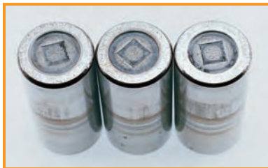
Roller end scoring — Metal-to-metal contact from breakdown of lubricant film.
