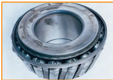
Cone large rib face deformation — Metal flow from excessive heat generation.
