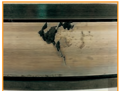
Point surface origin — Spalling from debris or raised metal exceeding the lubricant film thickness.
