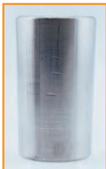
Roller nicking/denting — Rough handling or installation damage.
