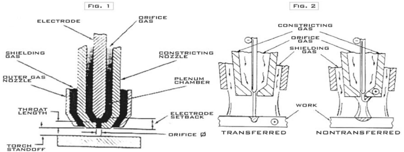
Electrodes of pure tungsten or tungsten with additions of thoria, zirconia or ceria are used with PAW. Direct current electrode negative (DCEN) is used for most applications since the heat generated is very high at the electrode tip, and when positive, the electrode will quickly deteriorate at currents in excess of 100 A. Pulsed current is often used. Operation on AC for oxide removal on aluminium or magnesium is possible, but here again, currents in excess of 100 A damage the electrode.
